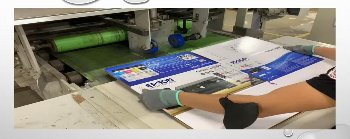
For semi-auto gluing process, operator's feedback was they do not encounter bloated on the creasing line when they folding the item.
